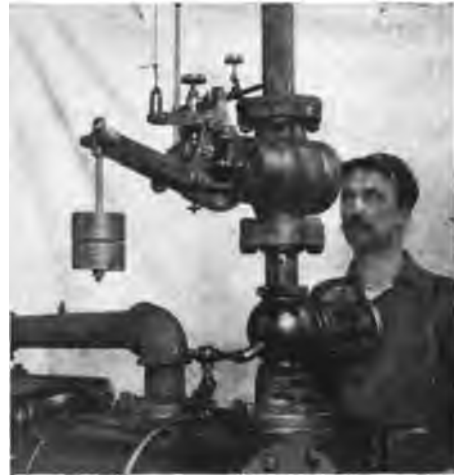
Fig. 2. Quick-Closing Piston Valve with Mechanical Trip.
